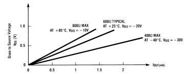
Figure 4. Output Impedance On
