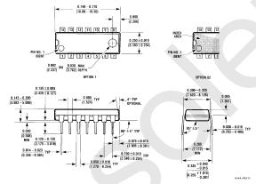
Molded Dual-In-Line Package (N) Order Number MM54C906N, MM54C907N, MM74C906N or MM74C907N NS Package Number N14A
