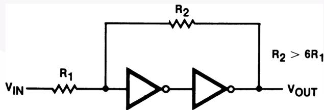
Figure 3. Schmitt Trigger
