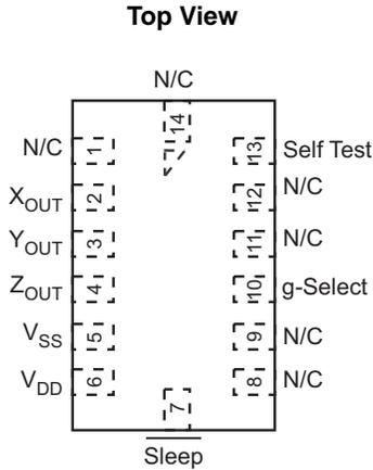
**Figure 4. Pinout Description**
