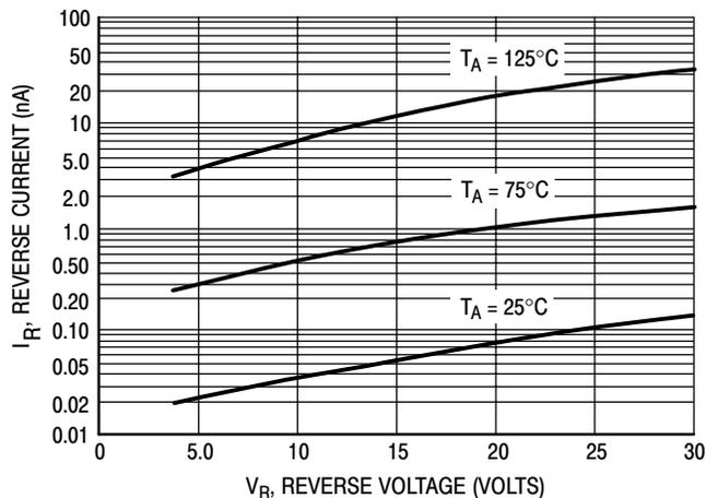
Figure 3. Reverse Current versus Reverse Bias Voltage
