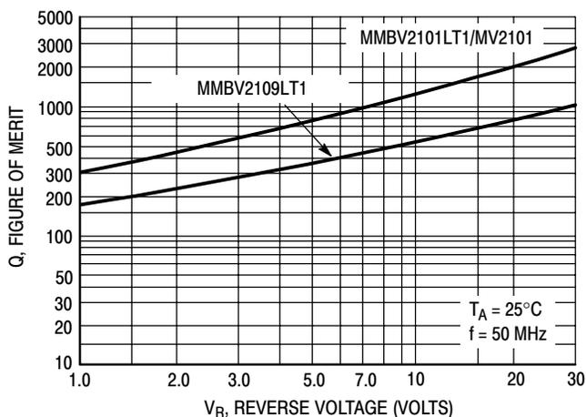
Figure 4. Figure of Merit versus Reverse Voltage
