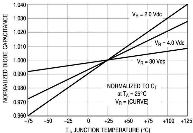
Figure 2. Normalized Diode Capacitance versus Junction Temperature
