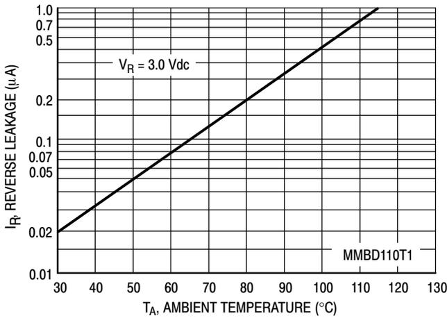
Figure 1. Reverse Leakage
