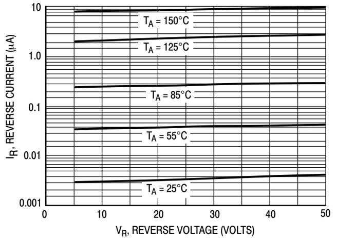
Figure 3. Leakage Current
