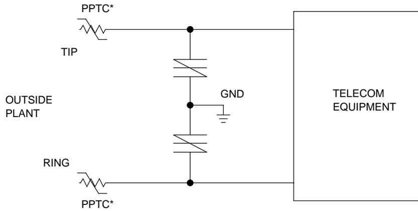
\*Polymeric PTC (positive temperature coefficient) overcurrent protection device
