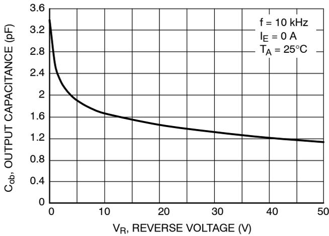
Figure 4. Output Capacitance
