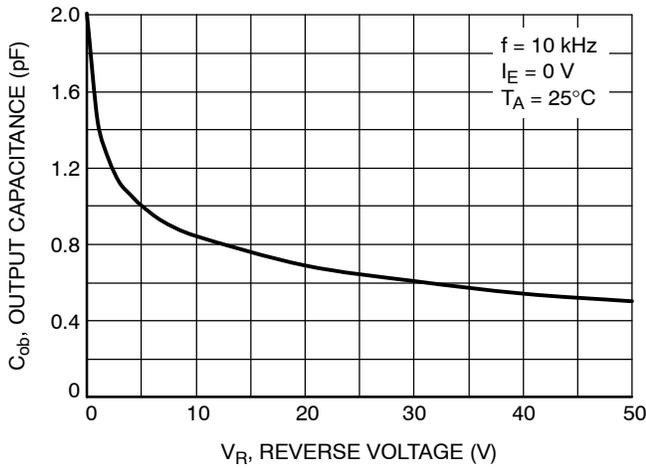
Figure 9. Output Capacitance
