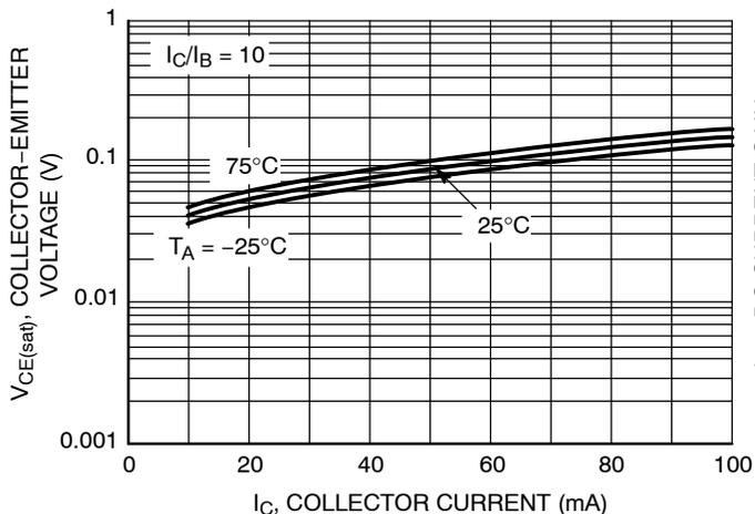
Figure 2.  $V_{CE(sat)}$  vs.  $I_C$
