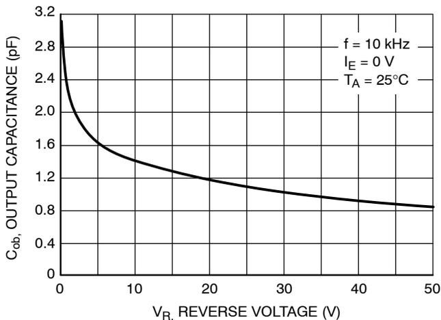
Figure 4. Output Capacitance
