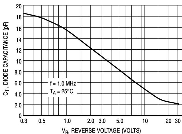
Figure 1. Diode Capacitance
