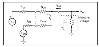
FIGURE 1. MPC506A Static Accuracy Equivalent Circuit.
