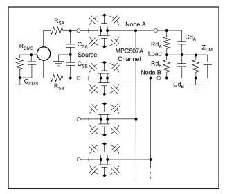
FIGURE 4. Settling and Common-Mode Effects—MPC507A
