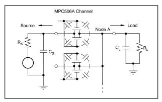
FIGURE 3. Settling Time Effects—MPC506A.
