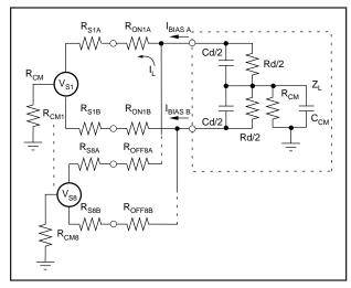
FIGURE 2. MPC507A Static Accuracy Equivalent Circuit.
