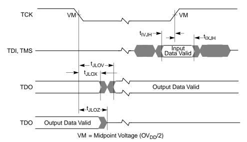
Figure 17. Test Access Port Timing Diagram
