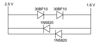
Figure 21. Example Voltage Sequencing Circuit
