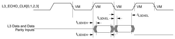
**Note:** t<sub>L3DVEH</sub> and t<sub>L3DVEL</sub> as drawn here will be negative numbers, i.e., input setup time will be time after the clock edge.
