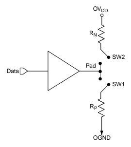
Figure 22. Driver Impedance Measurement
