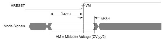
Figure 5. Mode Input Timing Diagram
