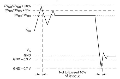
Figure 2 shows the undershoot and overshoot voltage on the MPC7450.
