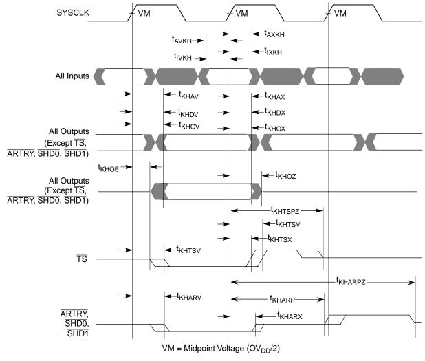
Figure 6. Input/Output Timing Diagram
