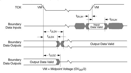
Figure 16. Boundary-Scan Timing Diagram
