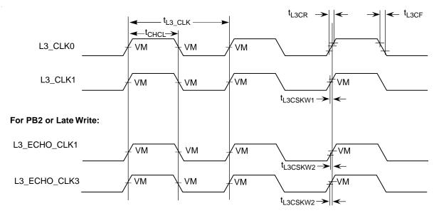
Figure 7. L3 CLK OUT Output Timing Diagram
