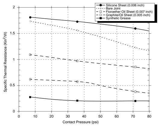
Figure 26. Thermal Performance of Select Thermal Interface Material
