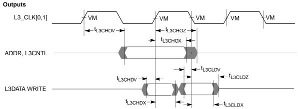
**Note:** t<sub>L3CHDV</sub> and t<sub>L3CLDV</sub> as drawn here will be negative numbers, i.e., output valid time will be time before the clock edge.
