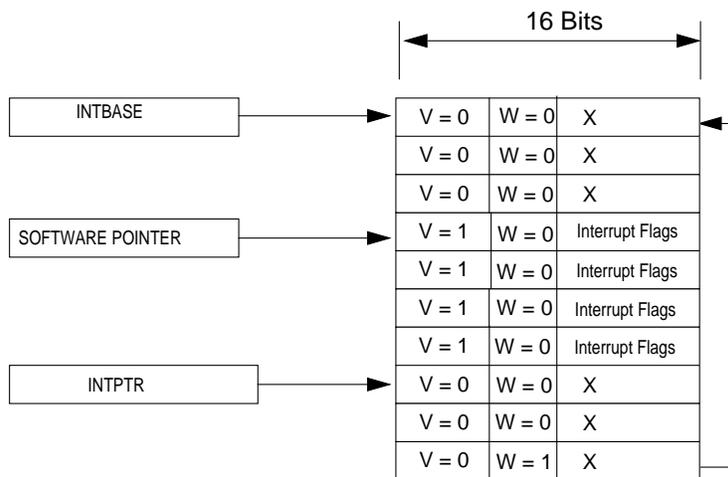
**Figure 4-1. Circular Interrupt Table in External Memory**
