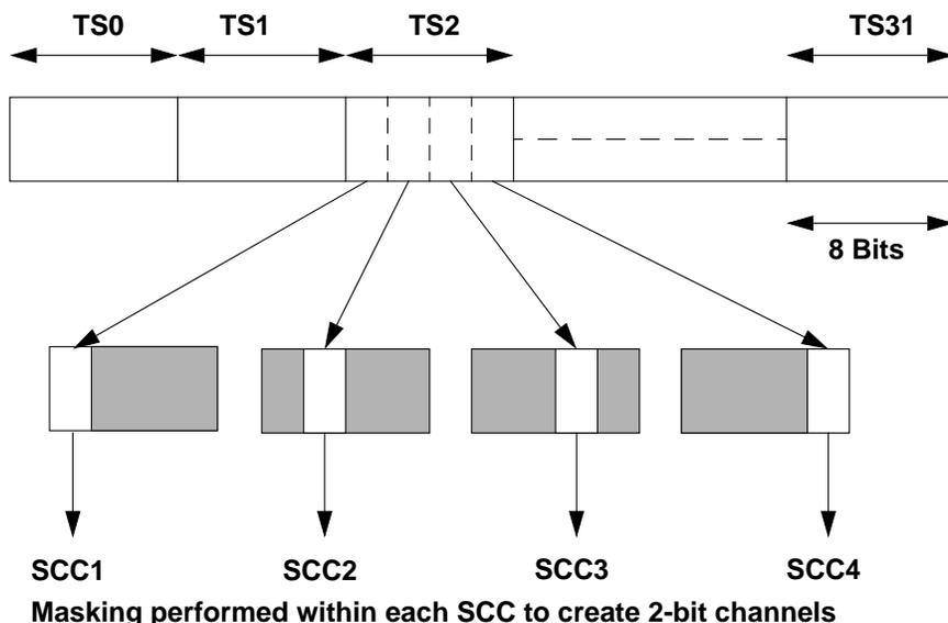
**Figure 9-1. Two-Bit Subchannel Implementation without MSC Microcode**
