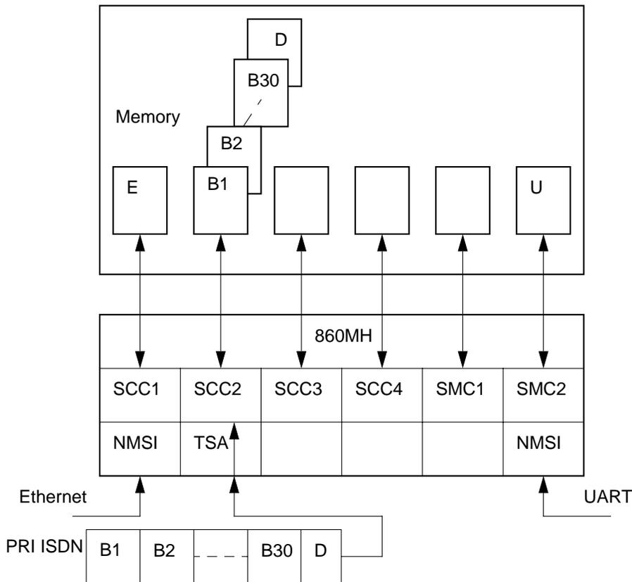
**Figure 1-7. Internal Routing for Ethernet-to-PRI Bridge Using MPC860**
