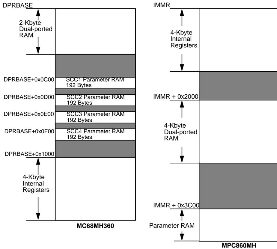
Figure 2-1. MC68MH360 and MPC860MH Internal Memory Structures
