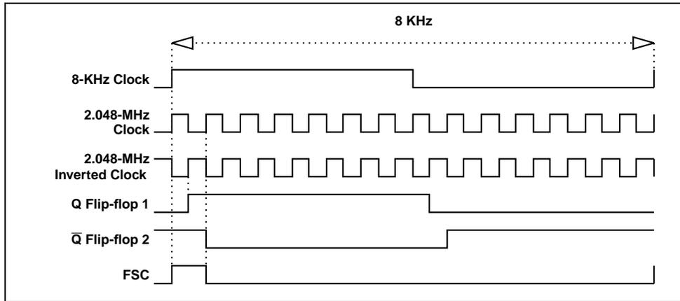
**Figure C-5. FSC Generation from a 2.048-MHz Clock—Timing**
