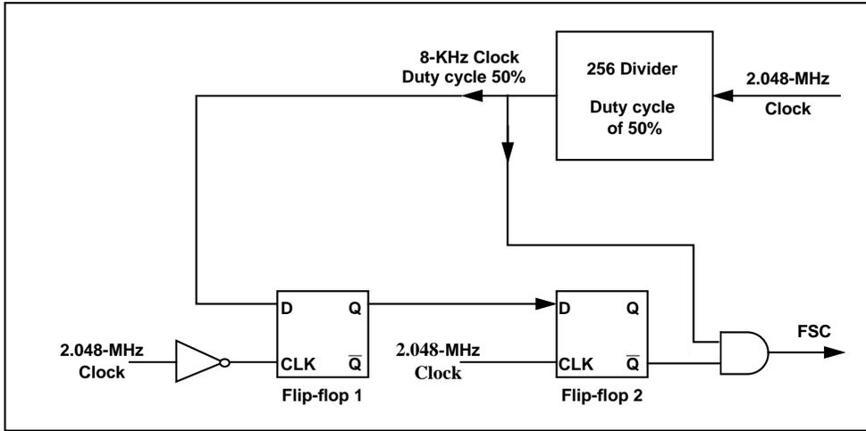
**Figure C-4. FSC Generation from a 2.048-MHz Clock—Block Diagram**
