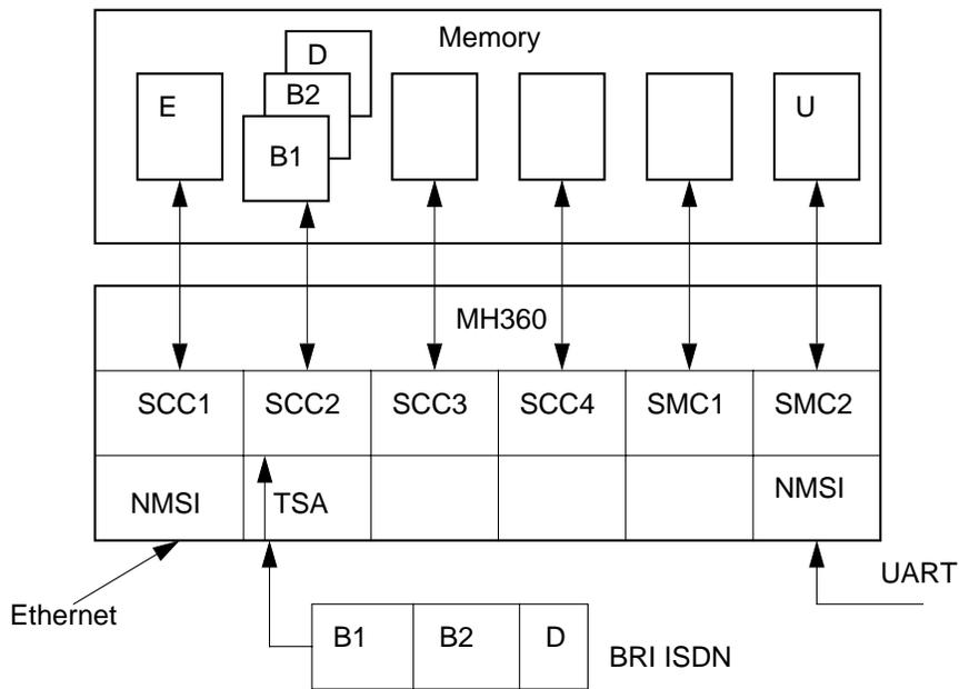
**Figure 1-5. Internal Routing for Ethernet-to-BRI Bridge Using MC68MH360**
