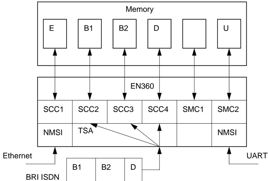
**Figure 1-3. Internal Routing for Ethernet-to-BRI Bridge Using MC68EN360**
