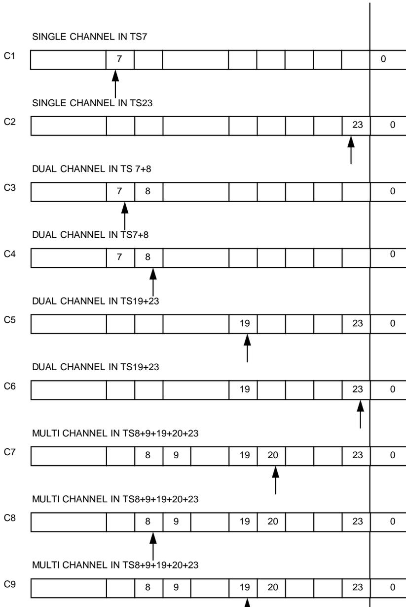
**Figure 2-14. Examples of Different T1 Time Slot Allocation**
