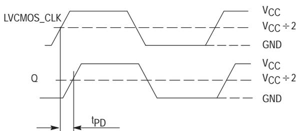
Figure 15. LVC MOS Propagation delay ( $t_{pD}$ ) test reference
