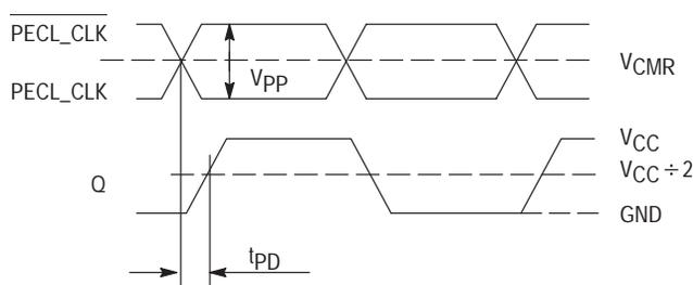
Figure 14. LVPECL Propagation delay ( $t_{pD}$ ) test reference
