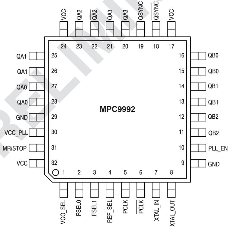
Figure 2. MPC9992 32-Lead Package Pinout (Top View)
