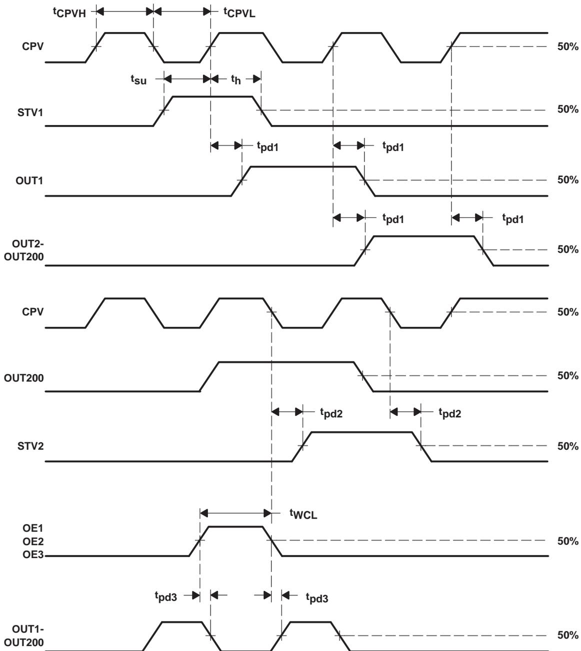
Figure 3. Timing Waveform
