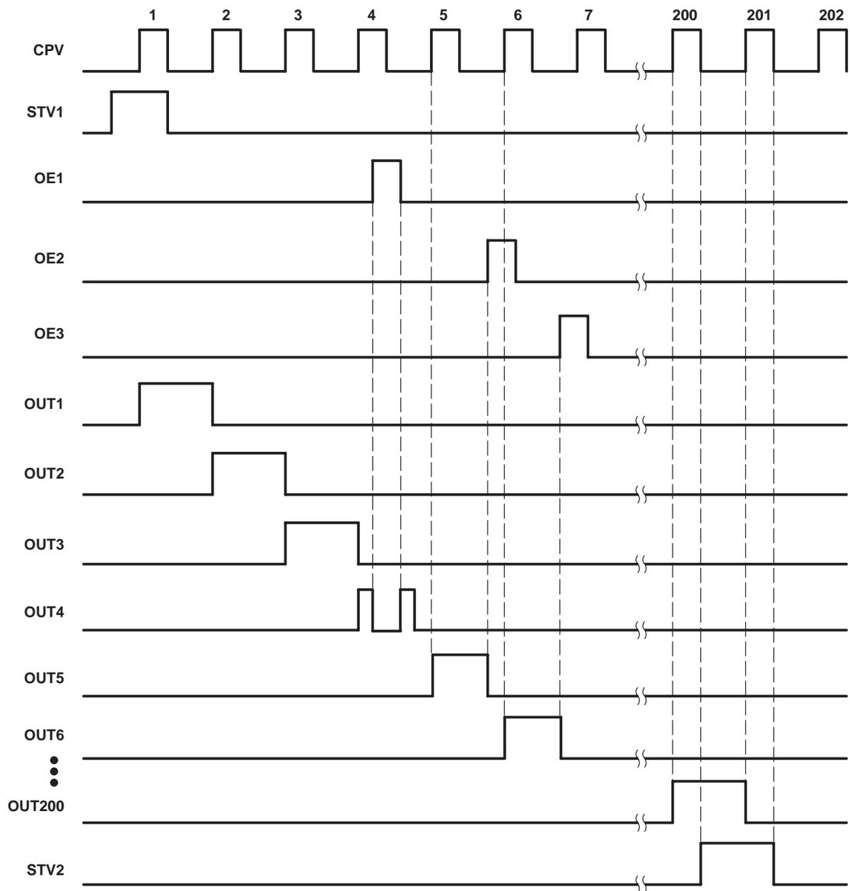
Figure 2. Recommended Operation Timing ( $L/\bar{R} = H$ )
