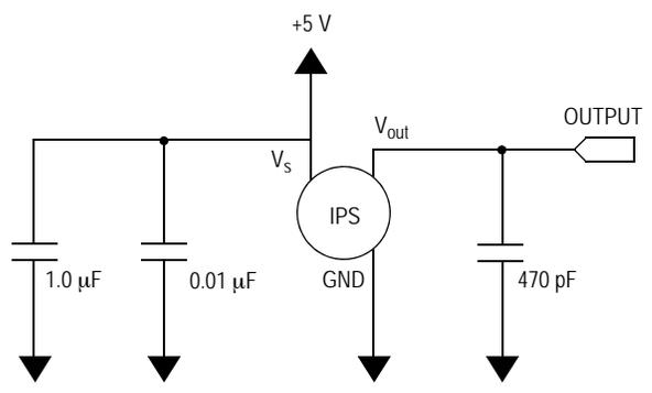
**Figure 3. Recommended Power Supply Decoupling and Output Filtering**
