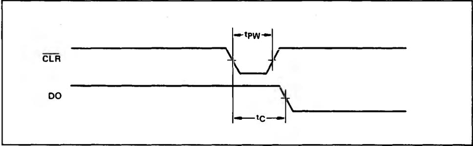
Output Buffer Enable/Disable (High Impedance Status) Operation
