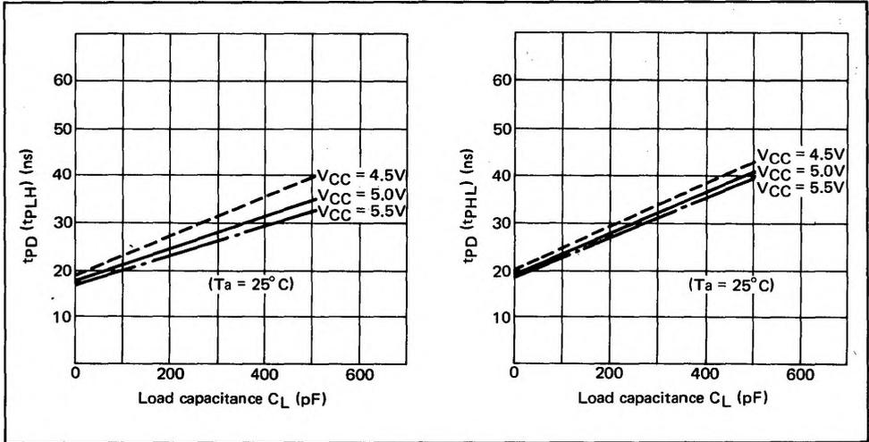
(2)  $t_{PD}$  and  $t_{WE}$  vs. supply voltage
