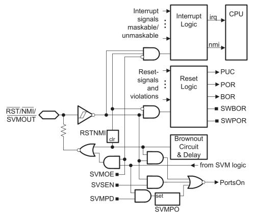
Figure 2. RST/NMI/SVMOUT and PortsOn Logic Block Diagram
