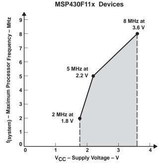
NOTE: Minimum processor frequency is defined by system clock. Flash program or erase operations require a minimum V<sub>CC</sub> of 2.7 V.
