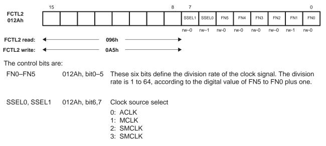
The flash timing generator is reset with PUC. It is also reset if the EMEX bit is set.
