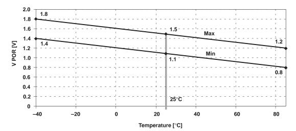
Figure 7. V(POR) vs Temperature
