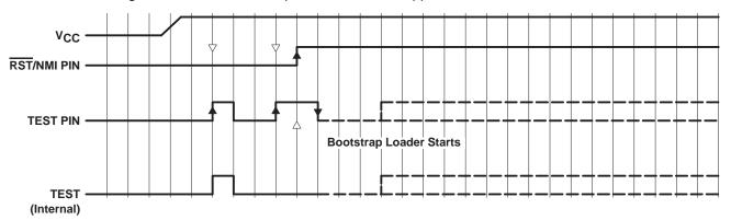
Test mode can be entered again after TEST is taken low and then back high.
