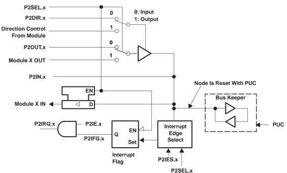
NOTE: x = Bit/identifier, 6 to 7 for port P2 without external pins
