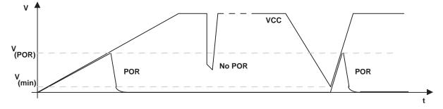
Figure 6. Power-On Reset (POR) vs Supply Voltage
