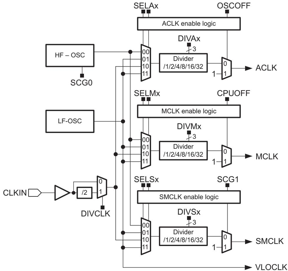
Figure 1. Compact Clock System (CCS) Block Diagram
