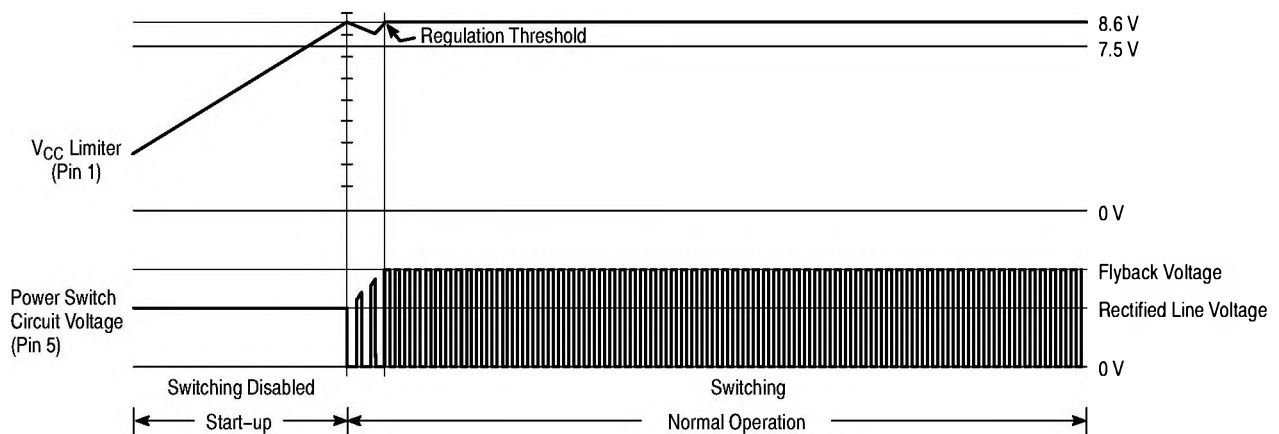
Figure 19. Start-up and Normal Operation Timing Diagram
