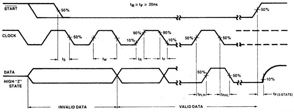
Propagation Delay Time  $t_p$  (Data)
