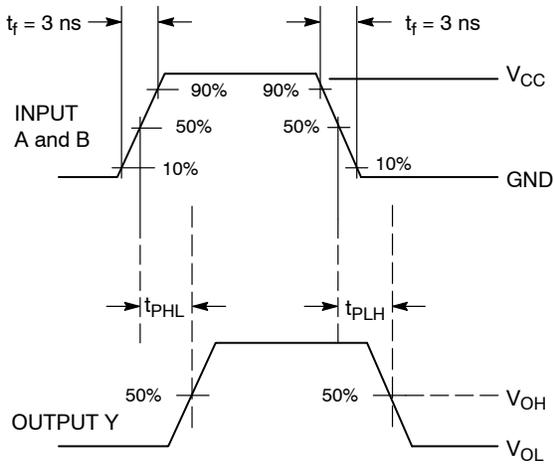
Figure 3. Switching Waveform
