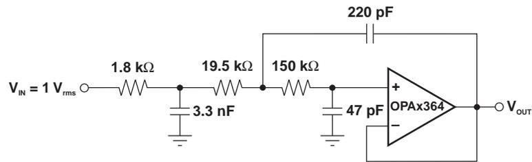
**Figure 29. OPAx364 Configured as 3-Pole, 20-kHz, Sallen-Key Filter**
