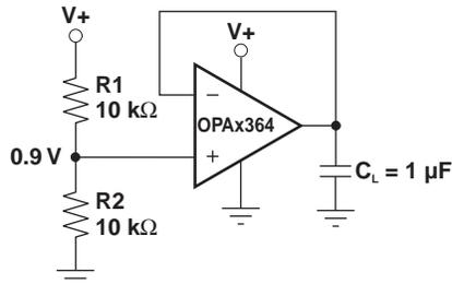
**Figure 25. OPAx364 Provides a Stable Reference Voltage**
