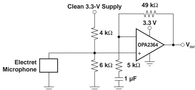
**Figure 28. Microphone Preamplifier**
