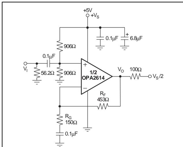
**Figure 3. AC-Coupled, G = +4, Single-Supply, Specification and Test Circuit**
