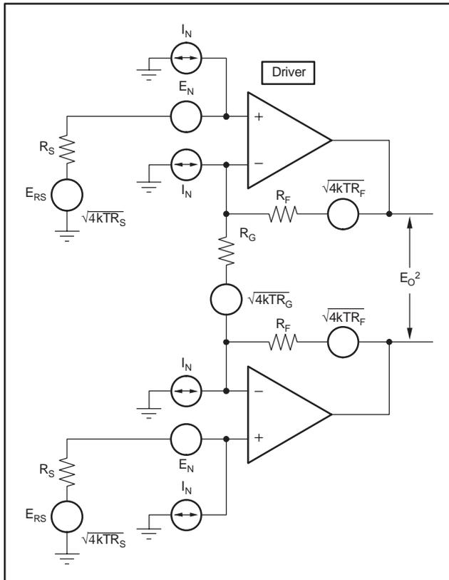
**Figure 18. Differential Op Amp Noise Analysis Model**
