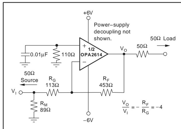
**Figure 14. Inverting Gain of –4 with Impedance Matching**
