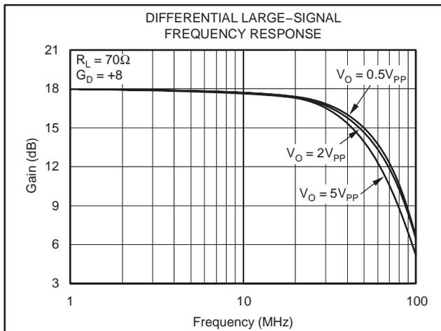
**Figure 7. OPA2614 Differential Gain of +8 Large-Signal Bandwidth**
