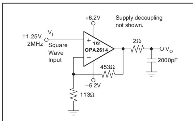
Figure 15. Large Capacitive Load Driver
