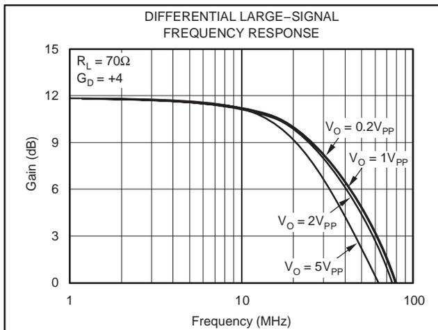
**Figure 6. OPA2613 Differential Gain of +4 Large-Signal Bandwidth**
