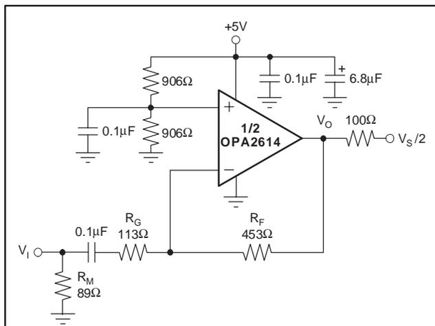
**Figure 4. AC-Coupled, G = -4, Single-Supply, Specification and Test Circuit**
