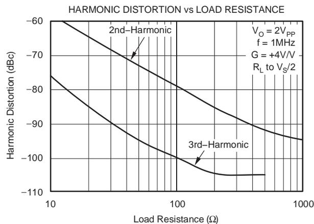
**TYPICAL CHARACTERISTICS:  $V_S = +5V$ , Differential Configuration**
