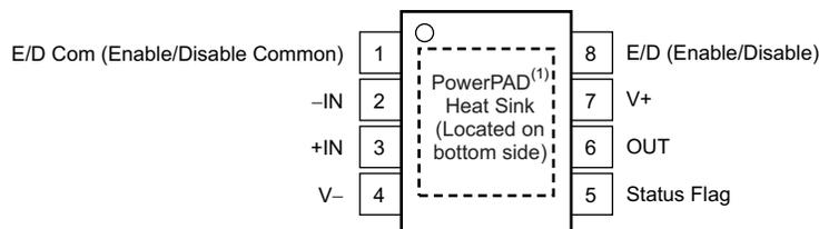
(1) PowerPAD is internally connected to V-. Soldering the PowerPAD to the printed-circuit board (PCB) is always required, even with applications that have low power dissipation.
