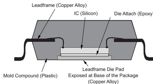
**Figure 84. Cross-Section View of a PowerPAD Package**
