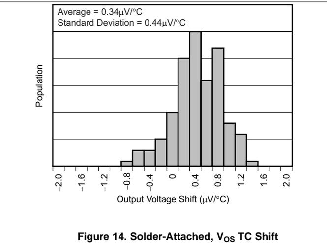
Figure 14. Solder-Attached,  $V_{OS}$  TC Shift
