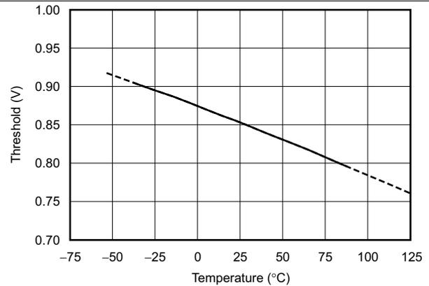
Figure 46. Enable/Disable Threshold vs Temperature
