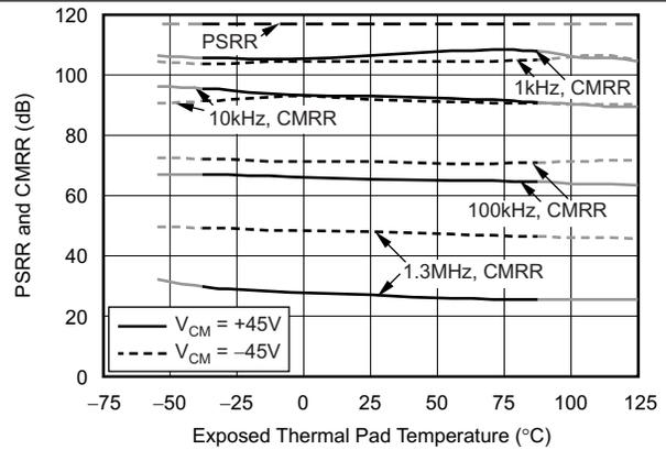
Figure 8. Power-Supply and Common-Mode Rejection Ratio vs Temperature
