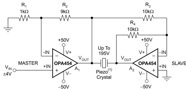
(1) For transducers with large capacitance, stabilization may become an issue. Be certain that the *Master* amplifier is stable before stabilizing the *Slave* amplifier.
