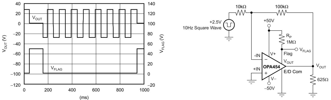
**Figure 86. Thermal Shutdown**
