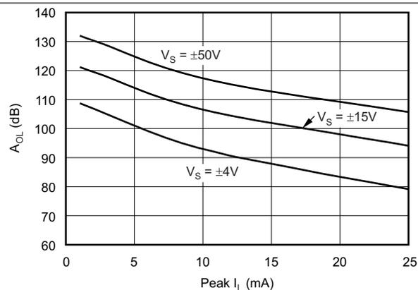
Figure 5. Open-Loop Gain vs Peak-Load Current
