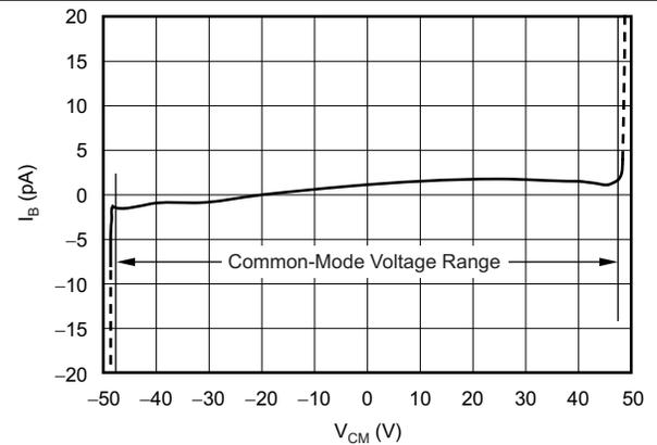
Figure 22. Input Bias Current vs Common-Mode Voltage
