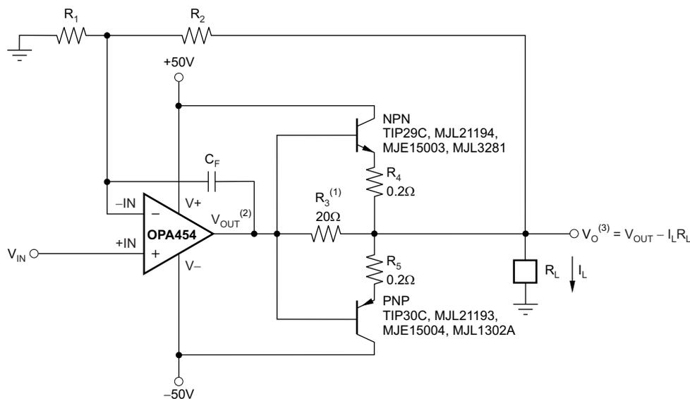
(1) Provides current limit for OPA454 and allows the amplifier to drive the load when the output is between +0.7 V and -0.7 V.
