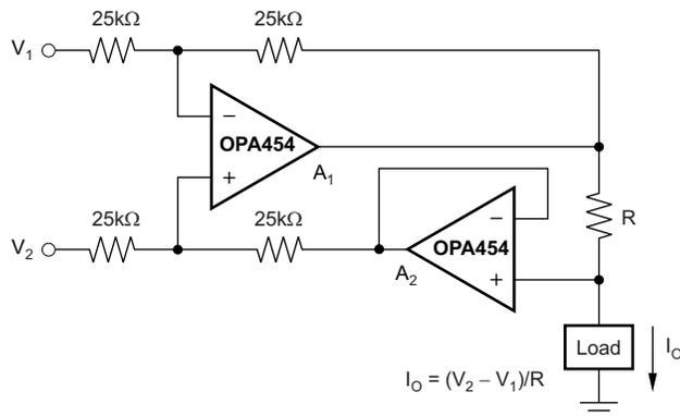
Figure 76. Differential Input Voltage-to-Current Converter for Low I<sub>OUT</sub>
