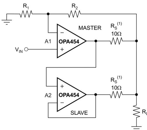
(1)  $R_S$  resistors minimize the circulating current that always flows between the two devices because of  $V_{OS}$  errors.
