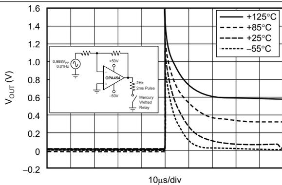
Figure 53. Remove Load (25-mA Source Response)
