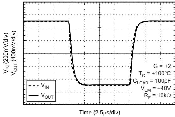
**Figure 33. Large-Signal Step Response**
