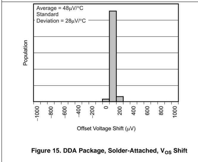
Figure 15. DDA Package, Solder-Attached,  $V_{OS}$  Shift
