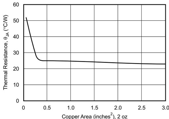
Figure 88. Thermal Resistance vs Circuit Board Copper Area
