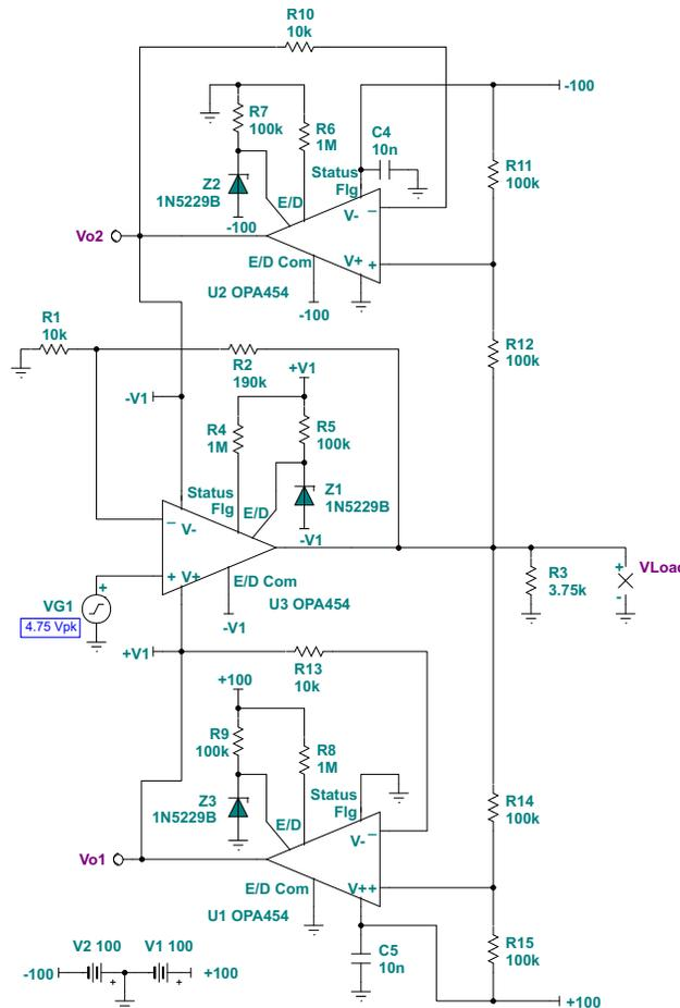
**Figure 67. OPA454 Noninverting,  $A_V = 20$  V/V, Output Voltage Boost**
