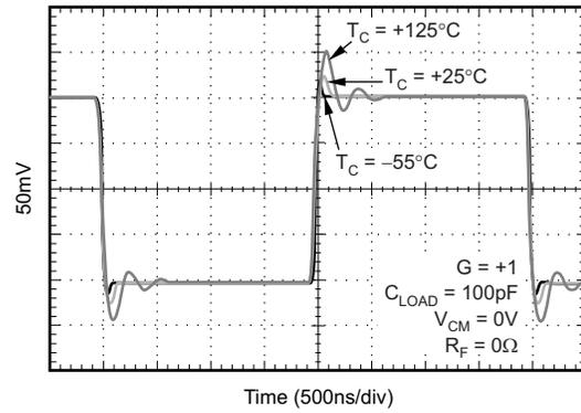
**Figure 34. Small-Signal Step Response**
