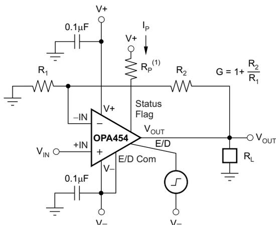
(1) Pullup resistor with at least 10  $\mu$ A (choose  $R_P = 1$  M $\Omega$  with  $V_+ = 50$  V for  $I_P = 50$   $\mu$ A).
