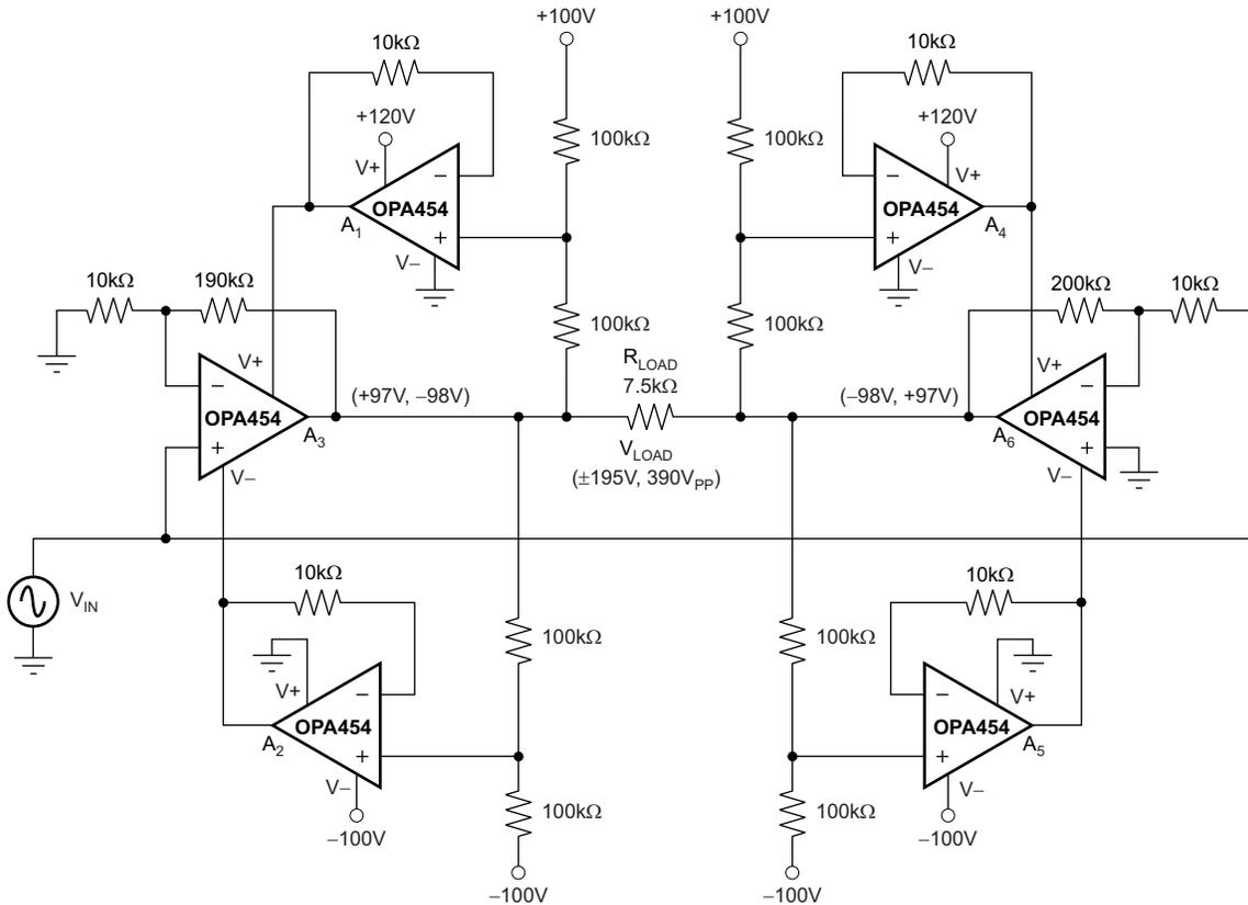
**Figure 81. Output Voltage Boost with ±195 V (390 V<sub>PP</sub>) Across Bridge-Tied Load (Six Op Amps, see Figure 82 and Figure 83)**
