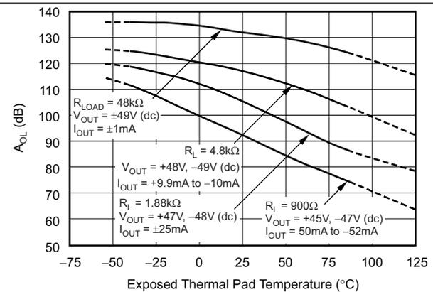
Figure 6. Open-Loop Gain vs Temperature
