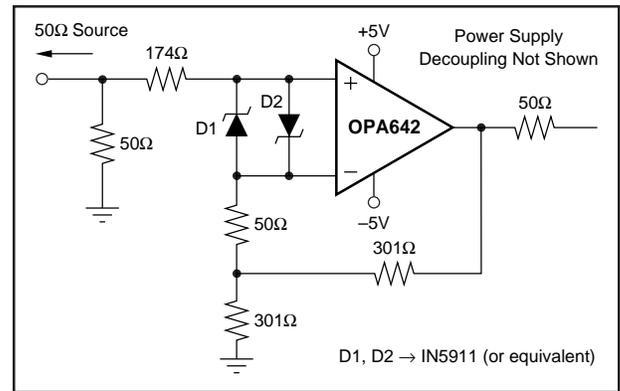
FIGURE 10. Gain of +2 with Input Protection.
