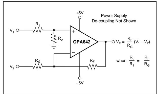
FIGURE 2. High Speed, Single Amplifier Differential Amplifier.
