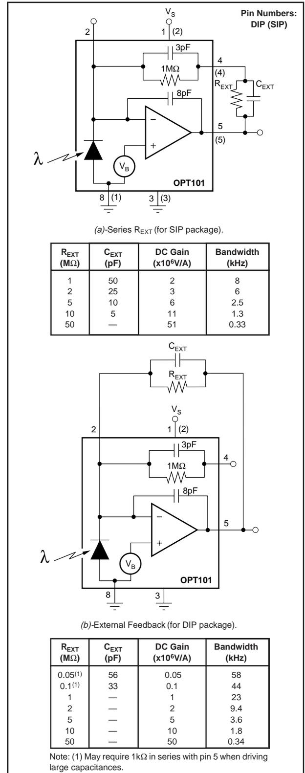
FIGURE 4. Changing Responsivity with External Resistor.
