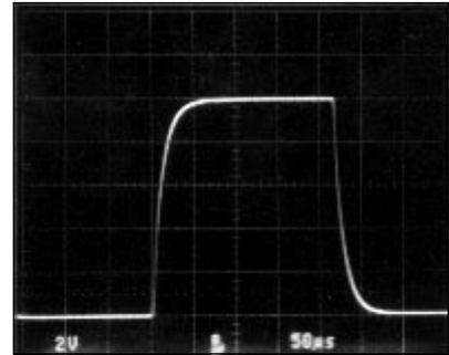
SMALL SIGNAL RESPONSE ( $C_{\text{LOAD}} = 10,000\text{ pF}$ )
