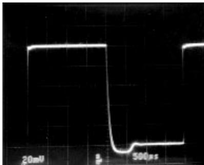
SMALL SIGNAL RESPONSE ( $C_{\text{LOAD}} = 10,000\text{ pF}$ )
