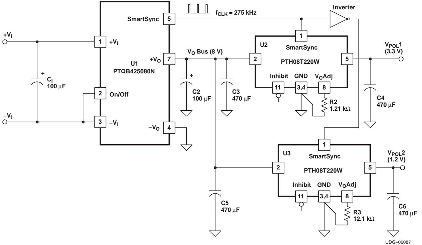
Figure 10. Synchronizing Modules Powered from the Same Bus
