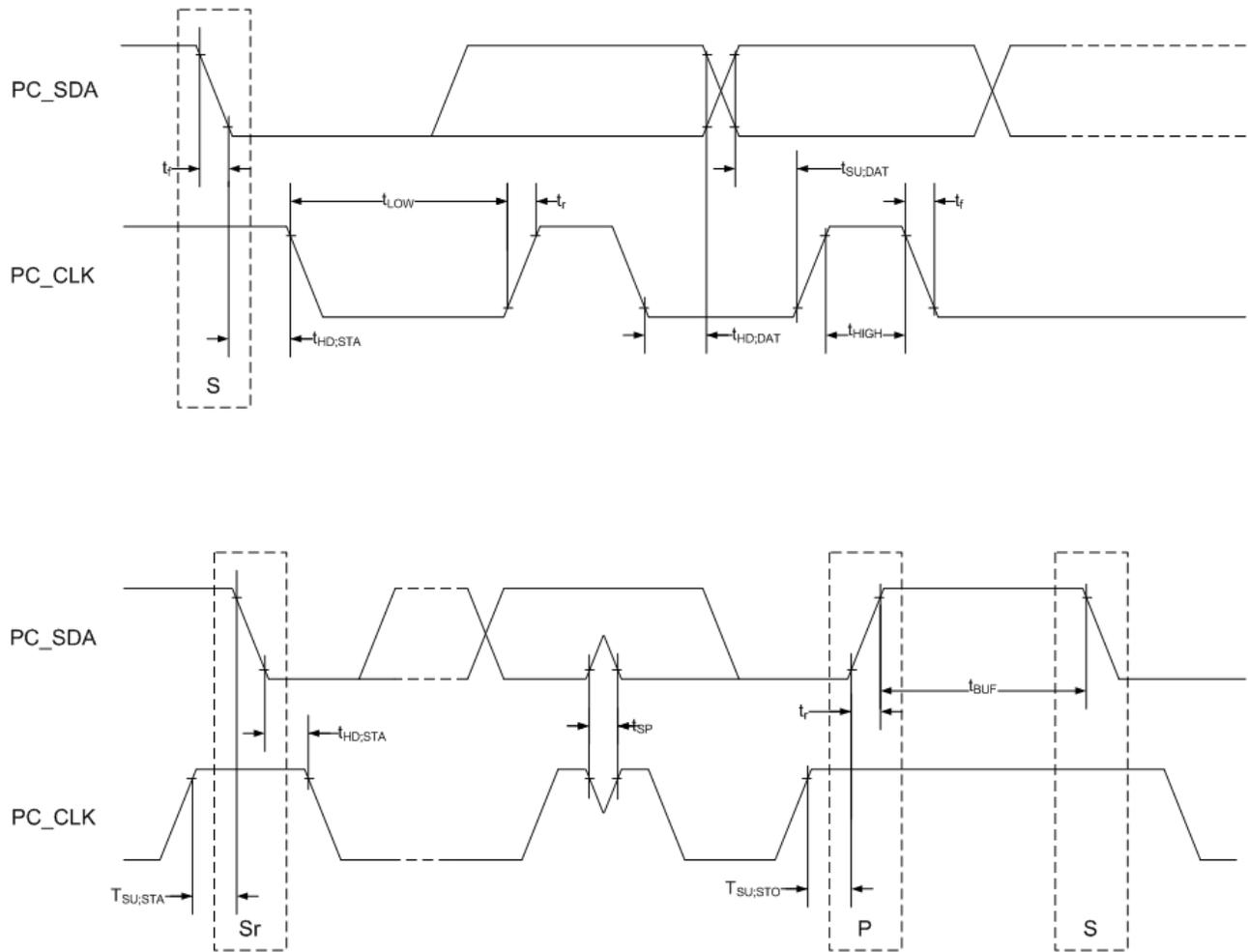
Figure 2. I<sup>2</sup>C Mode Timing
