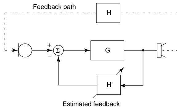
**Figure 5. Adaptive Feedback Canceller (AFC) Block Diagram**
