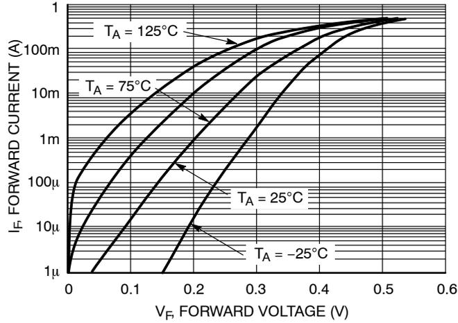
Figure 1. Forward Characteristics
