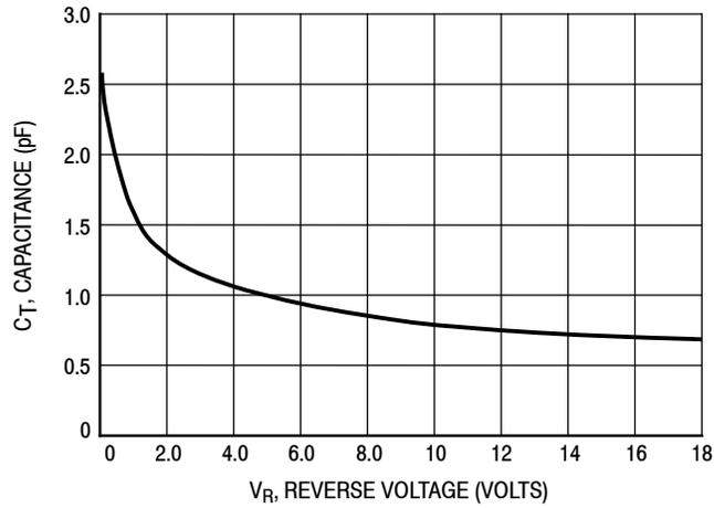
**Figure 4. Typical Capacitance**
