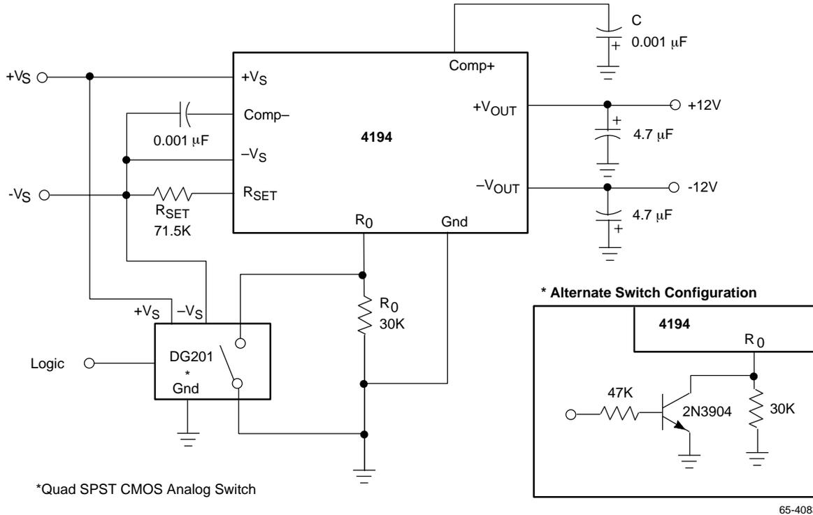
Figure 8.  $\pm 12$ V Switchable Power Supply
