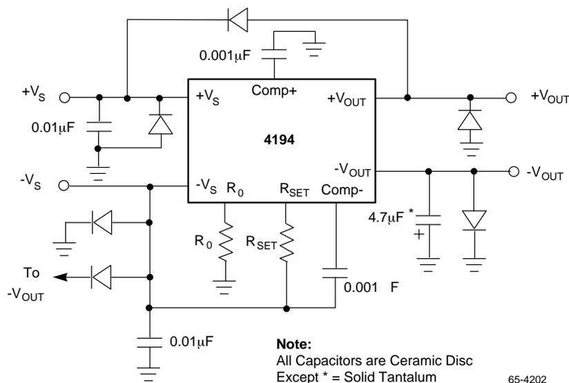
Figure 10. RC4194 Regulator Showing All Protective Diodes
