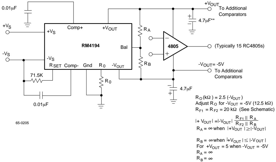
Figure 4. Unbalanced Output Voltage — Comparator Application
