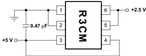
Figure 4. Typical Operating Connections for the REF3225
