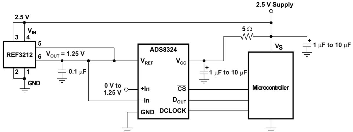
Figure 10. Basic Data Acquisition System 2
