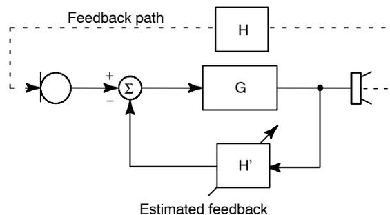
**Figure 6. Adaptive Feedback Canceller (AFC) Block Diagram**
