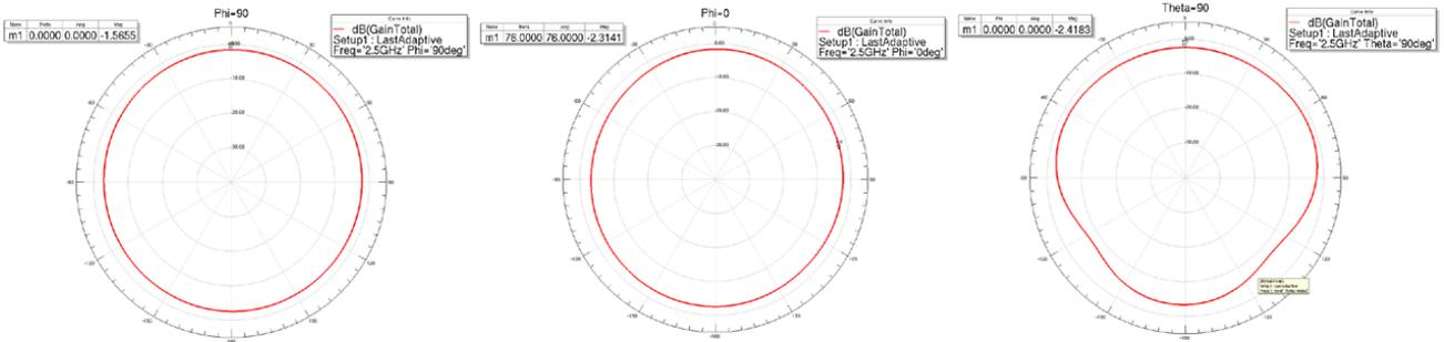
Figure 7. Radiation Pattern for PCB Ground Plane 2 (40 x 60 mm)
