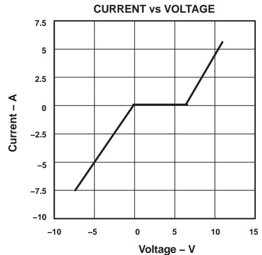
NOTE A: Typical current versus voltage curve was derived using the IEC 1.2/50- $\mu$ s surge waveform.
