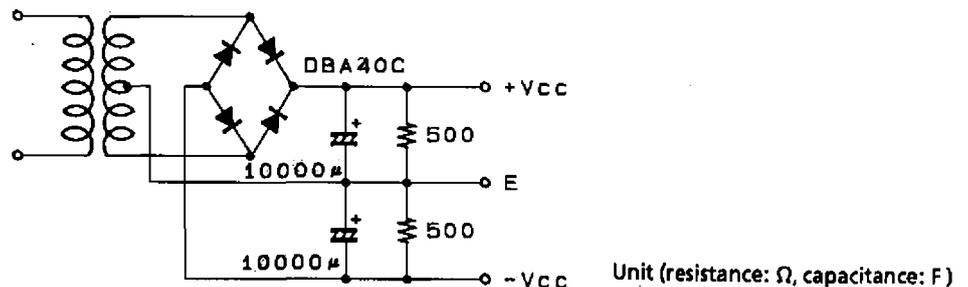
Specified transformer power supply (equivalent to MG-200)
