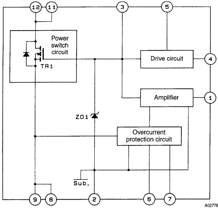
The back surface of the IC is not an insulator, and is effectively at pin 2 potentials
