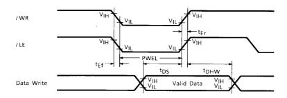
Test Conditions (1) ( $V_{SS} = 0 V$ ,  $V_{DD} = 3.0 V \pm 10\%$ ,  $V_{DD} - V_{EE} = 16 V$ , Ta = -20 to 75°C)
