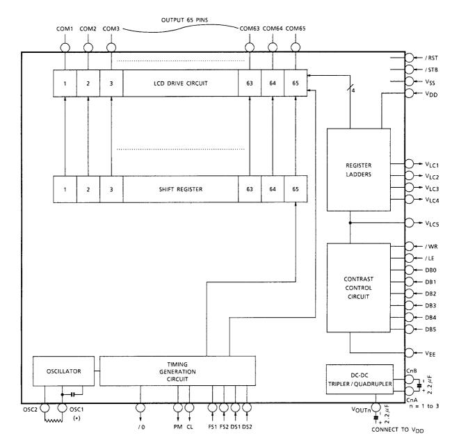
\*: When external clock operation is used, the clock should be input to OSC1.
