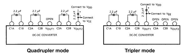
When not using the DC–DC converter, leave the CnA, CnB and VOUTn pins open and connect an external VEE supply.
