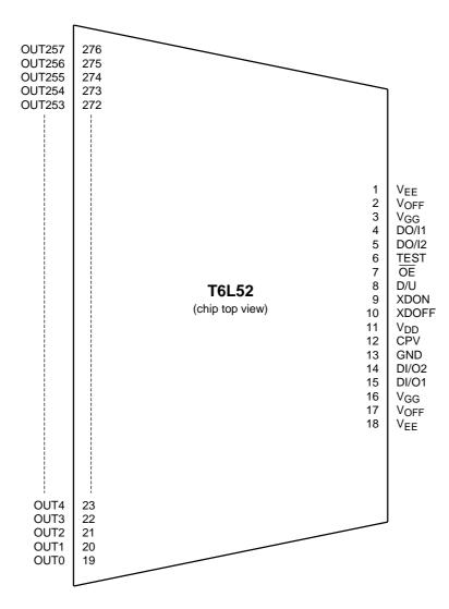
The above diagram shows the device's pin configuration only and does not necessarily correspond to the pad layout on the chip. Please contact Toshiba or our distributors for the latest TCP specification.
