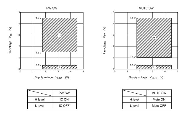
Figure 4 Switch sensitivity
