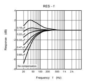
Figure 2 Capacitor response
