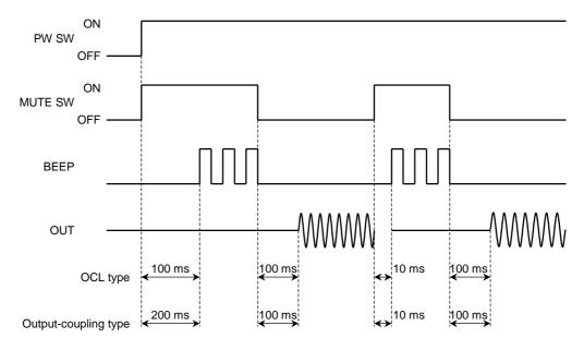
Figure 1 Timing chart for beep and output signals
