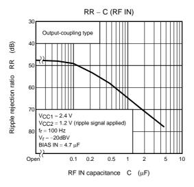
Figure 3 Improvement of ripple rejection ratio
