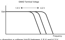
By changing a voltage (pin3) between 1.5 V and 4.2 V, frequency band width is changed.
