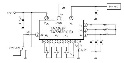
\*: Hall sensor driving current (I<sub>O</sub>) can be changed by I<sub>R</sub>. Refer to I<sub>R</sub> vs I<sub>O</sub> characteristics.
