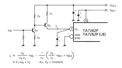
$Q_2$  works as a Current Regulator for Output Coil. Therefore, Collector to Emitter Voltage of  $Q_2$  is varied in accordance with required coil current.
