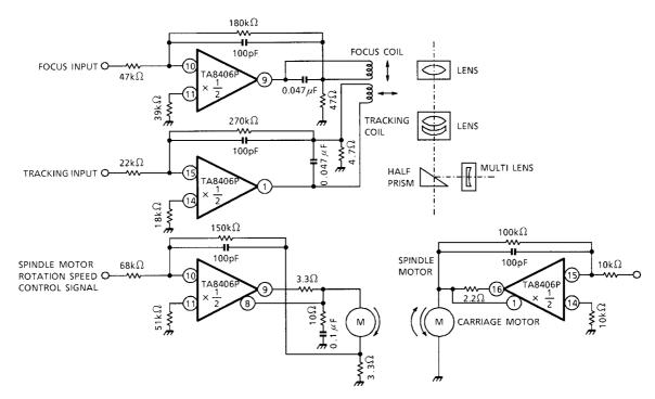
Note: Utmost care is necessary in the design of the output line, V<sub>CC</sub>, V<sub>EE</sub> and GND line since IC may be destroyed due to short-circuit between outputs, air contamination fault, or fault by improper grounding.
