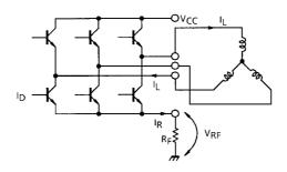
0 Torque state is obtained when less than 2.3 V of control voltage fed into input terminal. 0 Torque state also obtained by select a stop mode by controlling FRS input (Pin (4)). Less supply current is obtained with this condition.
