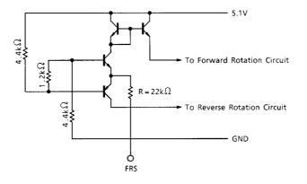
Forward, Reverse and Stop Modes are selectable by controlling this terminal. Specified voltages are less than 1.3 V (Forward), 2.4 $\sim$ 3.0 V or Open (Stop) and 3.9 V $\sim$ V<sub>CC</sub> (Reverse). VFRS – IFRS characteristic is shown below.
