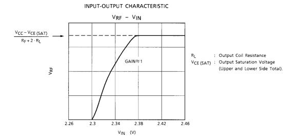
$V_{RF}$  is feed back voltage generated by  $R_{F}$  and output current of IL, drive current of ID and internal reference circuit current of IR. But IO and IR are negligible therefore,
