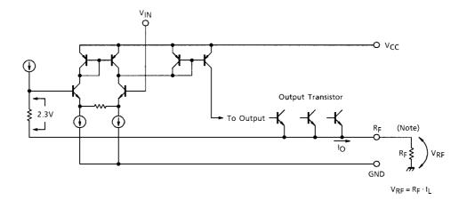
$V_{RF}$  (=  $R_{F} \cdot I_{L}$ ) of feed back voltage is feed backed to negative input of control amp internally. Voltage gain becomes approximately equal to 1 (0dB) by this internal feed back.
