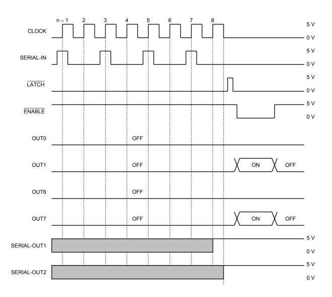
Note 2: The latches circuit holds data by pulling the LATCH terminal Low.
