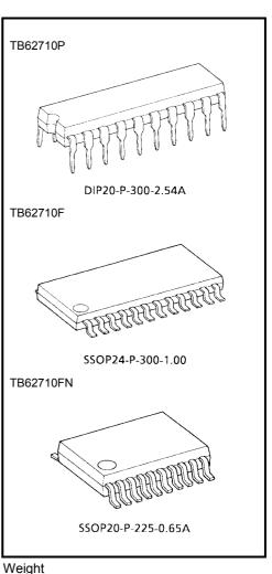
Weight DIP20-P-300-2.54A: 2.25 g (Typ.) SSOP24-P-300-1.00: 0.33 g (Typ.)
