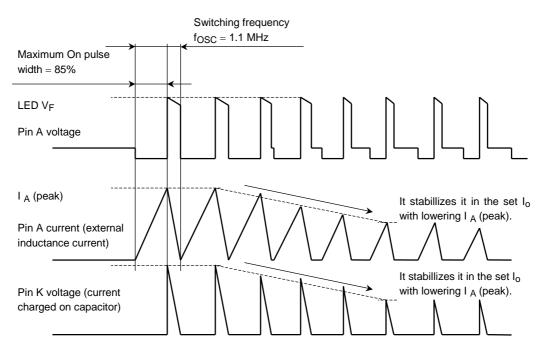
Figure 3 Burst Control Waveforms
