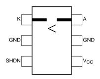
Note 1: Be careful of handling because there is a terminal which is poor at ESD in this product. This IC sometimes breaks when it is mounted at 180 degree for the reversal. Mount a circuit board in the accurate direction.
